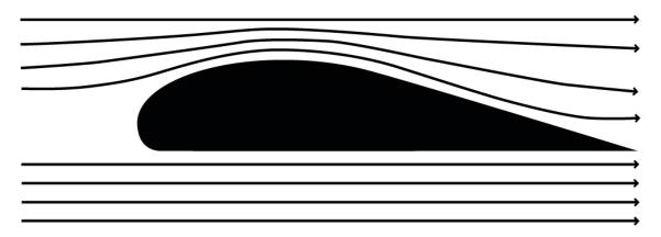
Airfoil is the name for the special shape of airplane wings. Wings come in different shapes and sizes, but a wing's airfoil shape—like a teardrop on its side—is always designed to create lift. An airplane wing is designed so air flows faster over the wing than it does beneath the wing.
